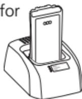
The red 'Charging' LED glows to indicate that the battery is charging.
